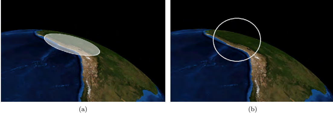
Figure 5.4: (a) The lens is represented as a circle over the globe, hence the lens' shape is not distortion-free. (b) Our adopted approach: the lens is a circle in 2D screen space.
